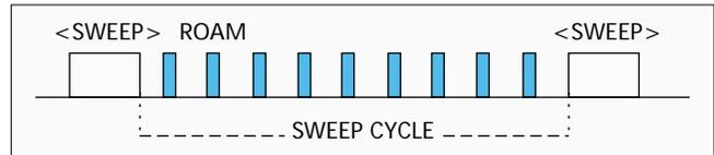
■ Figure 10. The roaming signals on a system channel.
