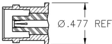
and C connectors. The BNC is essentially a miniature version of the C connector which is a Bayonet version of the N connector. BNC connectors are available in both 50 and 75 ohm versions, both versions will mate together. The 50 ohm designs operate up to a frequency of 4 GHz. BNC connectors are used in many applications, some of which are flexible networks, instrumentation and computer peripheral interconnections.
